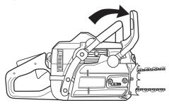
**Ignition; choke (A):** Pull out the blue choke control to the choke position. This should automatically set the red stop switch to the start position (upwards).
